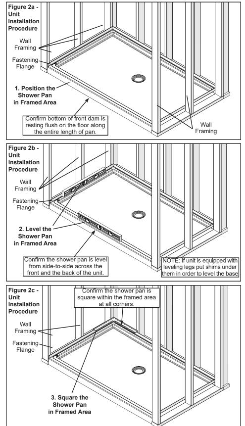
CAUTION: It is advisable to protect the unit surface with a thin plywood or cardboard shield while fastening the flange to the framing.
